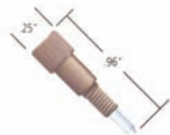
UP-M-645 6-40 PEEK/Kel-F™ Fitting for 1/32" OD tubing Max Pressure 121-224 bar
