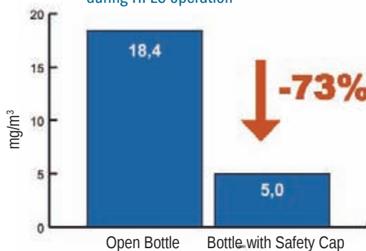
Emissions of Acetonitrile in a test laboratory during HPLC operation
