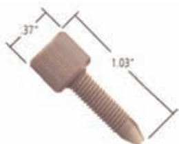
UP-F-130 10-32 PEEK™ Fitting Max Pressure 414 bar
