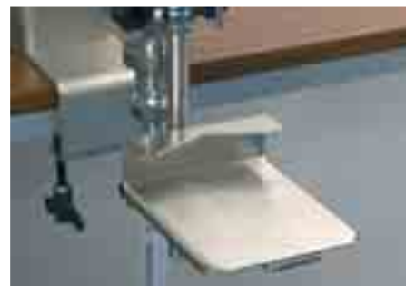
Variable filling table with centering device
