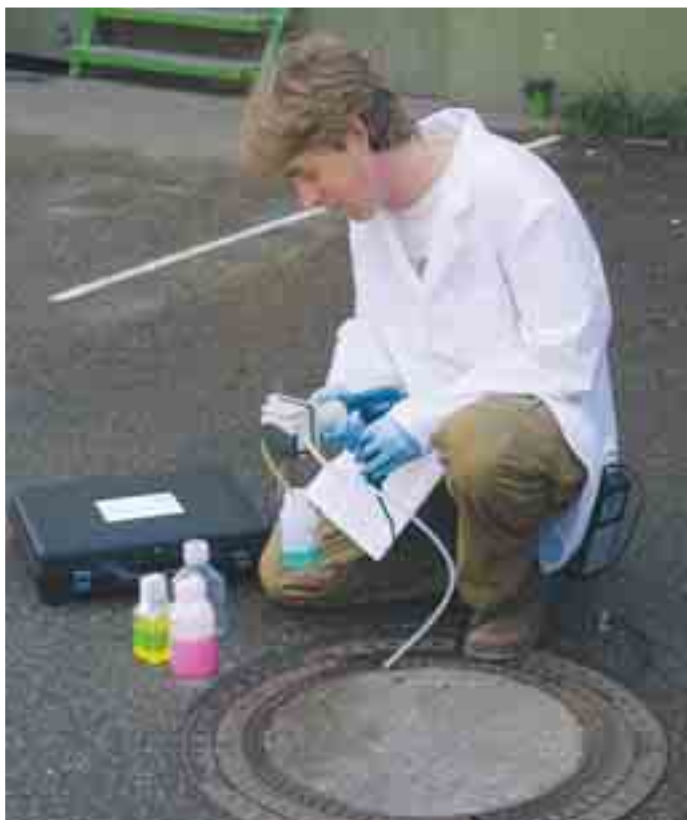
Vampire in use in the environmental protection sector for sampling from narrow openings and at substantial depths.
