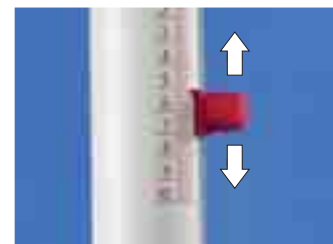
Set the required volume to be added with the adjustment screw
