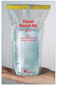
The samples of potable water to be used for microbiological testing need to be added of sodium thiosulfate to neutralize chlorine.
