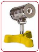
The sterilisation of metal inoculating loops and needles is a process that is daily performed in each clinical microbiological laboratory. The traditional flaming of Bunsen burner produces aerosol contamination on the bench with biohazard risk for the operator. The electrical sterilization performed using the "Bacteria Safe" from International PBI is ideal for labs and bio-safety cabinets avoiding the use of open flame. The sterilization of the metal inoculating loop and needle is obtained
