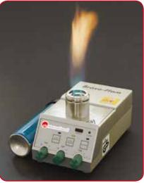
the risk of fire and gas explosion: the gas flows and ignites only if consciously activated. If the flame is accidently distinguished, the gas valve closes and prevents gas leaking. The "Bravo-Flam" works with a re-chargeable battery pack and is switched on without matches; the optical or foot switch give the possibility to operate with hands-free.
