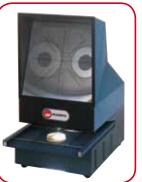
The method to evaluate the antibiotic potency of the drug is based on the production of an inhibition zone on the surface of a nutrient agar that incorporates a micro-organism. This test is performed using the traditional Petri dish or a large square plate for the "latin square" method.
